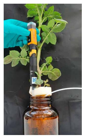
Measuring the pH value using WTW IDS wireless sensors in a potato plant
